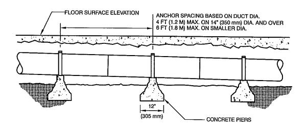
TYPICAL ANCHORAGE OF DUCTS TO BE ENCASED IN CONCRETE
